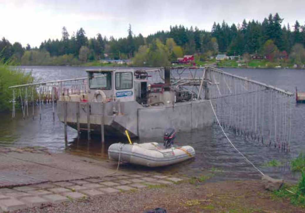
Figure 3. Alum application barge used at Long Lake, Kitsap County, Washington, April 2007.
