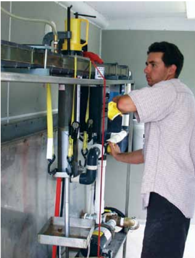
Figure 4. Sediment erodibility testing using a Mobile Adjustable Shear Stress Erosion and Transport (ASSET) Flume taken 7/13/2005. Pictured is Jesse Roberts, SNL.
