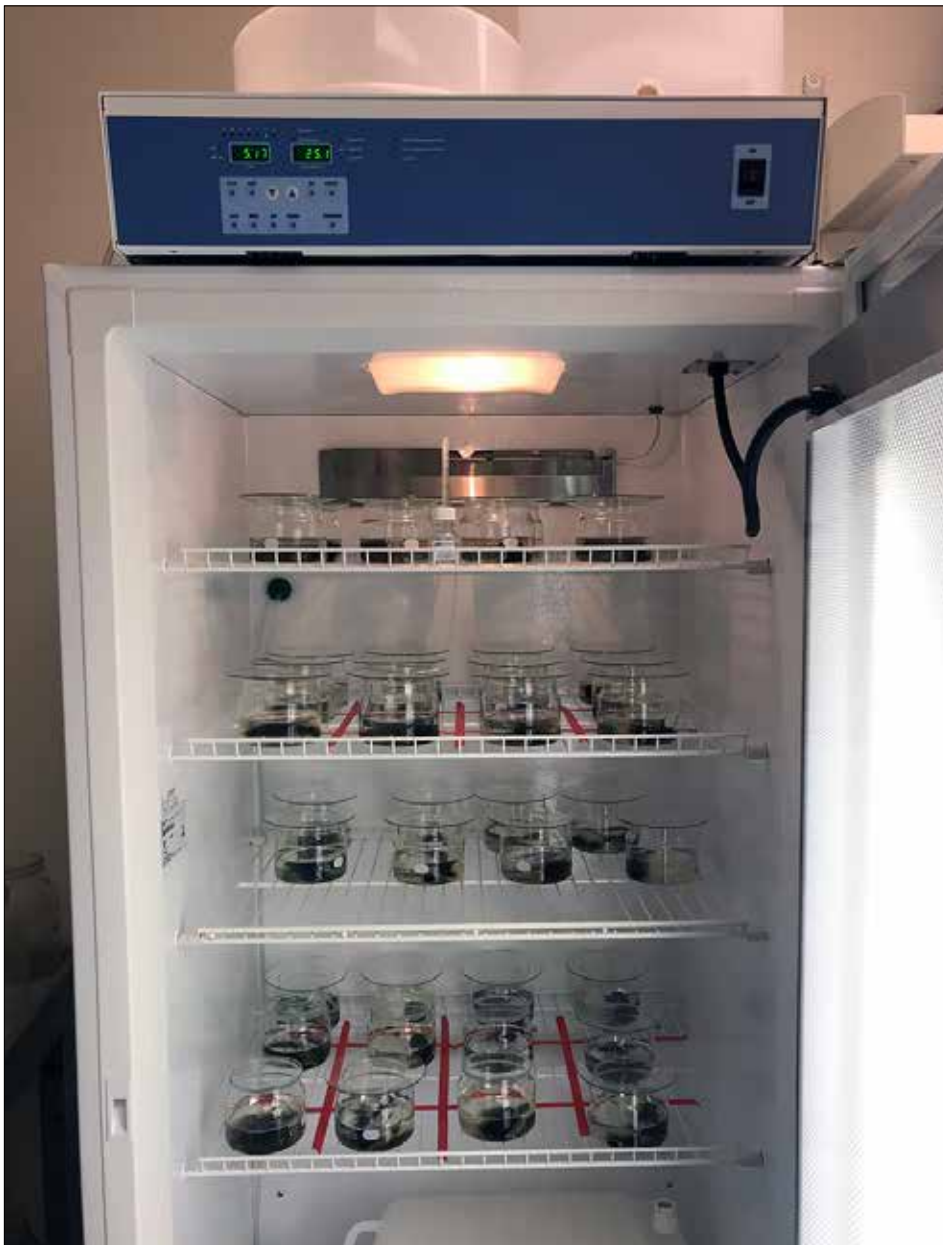
Figure 3. Treatment samples acclimating in an incubator set to 25 °C with a 16-hour light, 8-hour dark photo period. Photo credit: E. Vulgamore.
